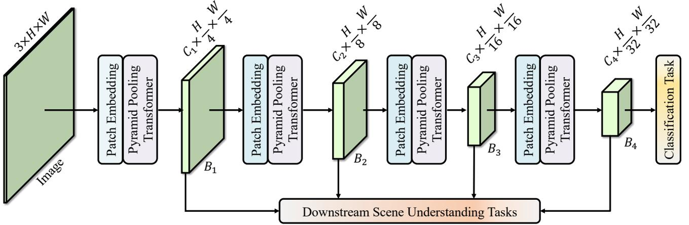
Fig. 2. **Architecture of the proposed P2T network.** We replace the traditional MHSA with our pooling-based MHSA. The feature maps  $\{B_1, B_2, B_3, B_4\}$  can be used for downstream scene understanding tasks.
